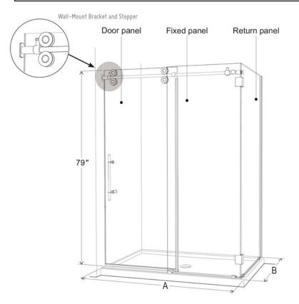
Minimum clearances required for glass panels sitting on a base threshold: 1/2" from the center of the glass panel to BOTH the exterior and interior sides
