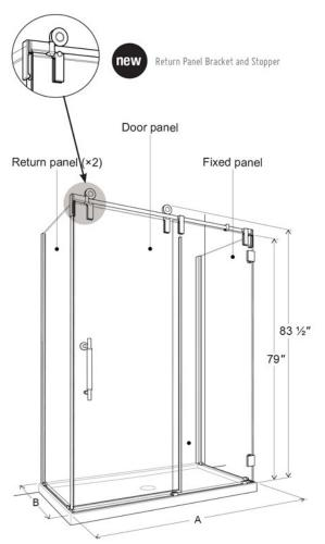
Minimum clearances required for glass panels sitting on a base threshold: 1/2" from the center of the glass panel to BOTH the exterior and interior sides
